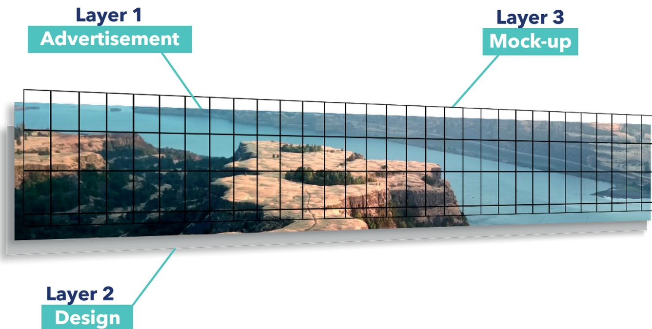
Mullion mock-up should be overlaid on the design to ensure appropriate treatment of advertising material. With the mock-up in place, it is easier to arrange the key items in relation to mullion grid.
